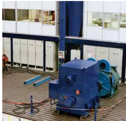
Motor MTK 560 (IP56), diesel electric marine propulsion
