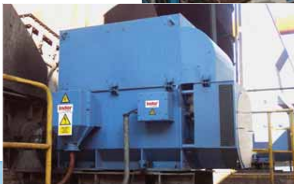
Tension reel motor in lamination plant
