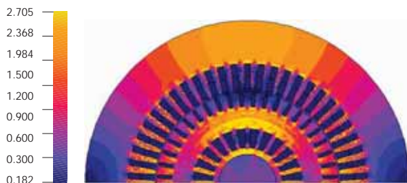
— Analysis of the distribution of magnetic induction carried out using finite element
