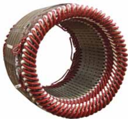
Medium voltage stator assembly ready to be introduced in the VPI tank
