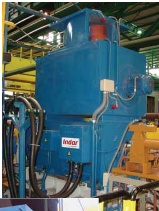
Tension reel motor in lamination plant
